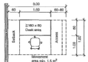
2 Minimum space requirement for a single workstation
