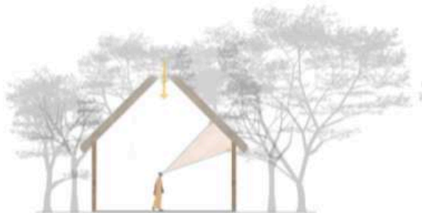
The negative impact of closed roof on ventilation and visual connection
