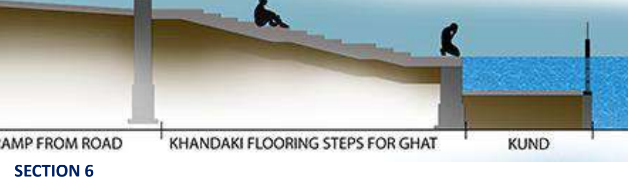
SECTION 6: REPAIRED BASALT STONE WALL, PROMENADE, ENTRY, PATHWAY, RAMP FROM ROAD, KHANDAKI FLOORING STEPS FOR GHAT, KUND
