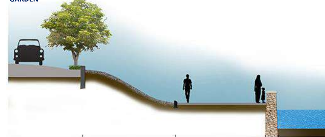
SECTION 1: ROAD, STONE PITCHING, PROMENADE, REPAIRED BASALT STONE WALL
