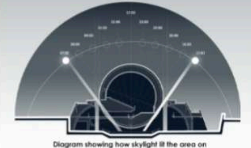
Diagram showing how skylight fill the area on different timings of the day.
