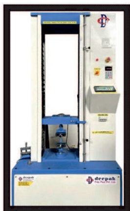
Figure 2 : Thermoplastic Sheet Specimen Being Tested For Tensile Strength
