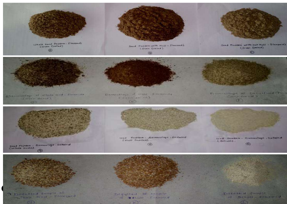
Fig. 3: Fractionating flaxseed parts separating lignan rich fraction
